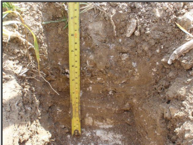
Plate 17 : Soil Profile 2 at TH11 - agricultural soil (calcareous)
