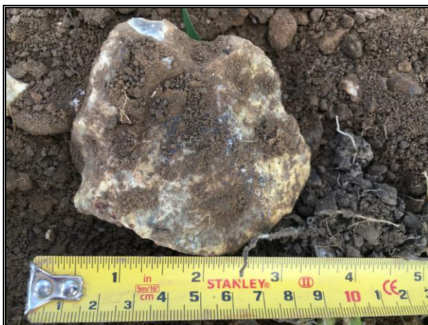
Plate 13: Soil Profile 1 – Sub-angular flint
