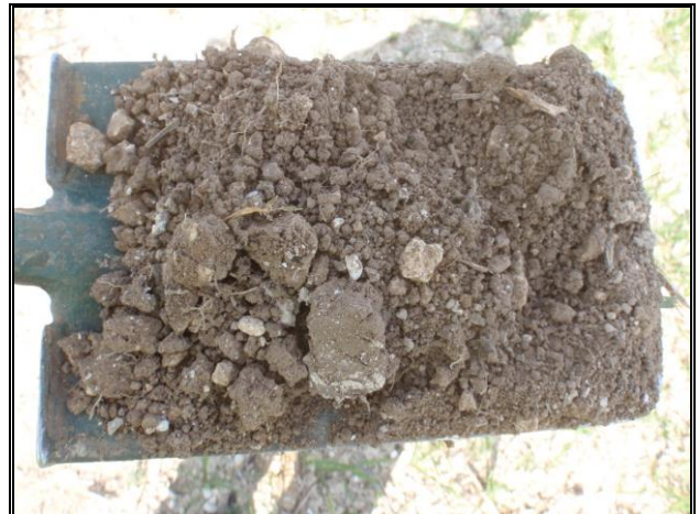
Plate 18 : Topsoil 2 arisings - agricultural soil (calcareous)
